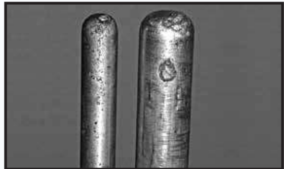
Blunt rods were struck by lightning
