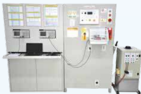
Lightning Impulse Current Test 60kA, 10/350 \mu s & 8/20 \mu s
